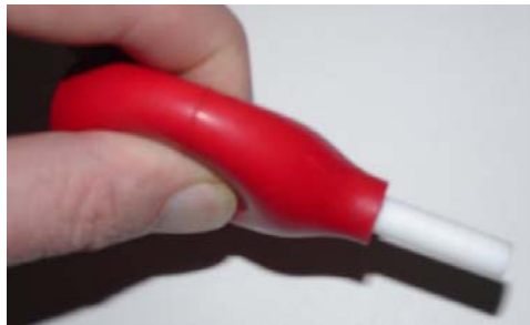
Figure 6, Rotor removal suction bulb.
