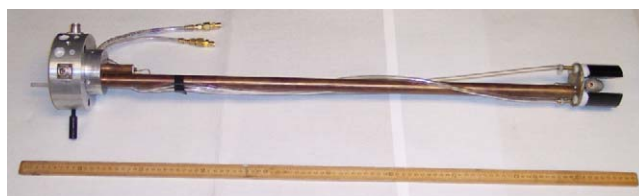
Fig. 8. Photograph of prototype 3\lambda/4 coax probe, with a 7 mm OD MAS module.
